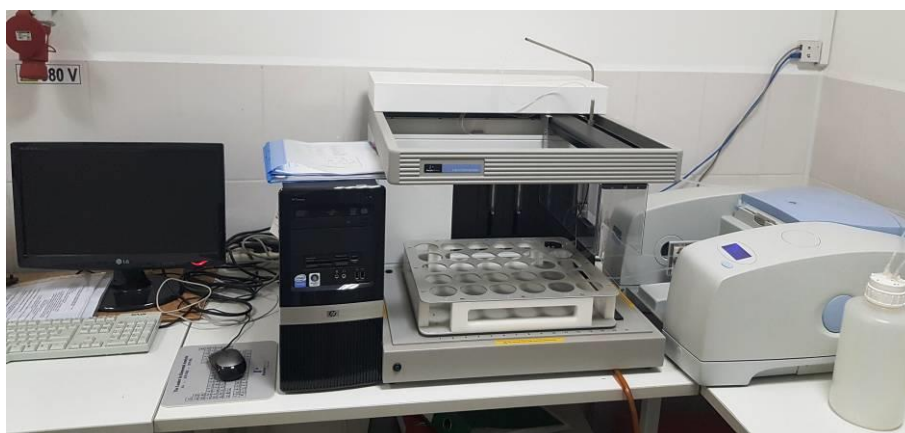
Fig. 4. Perkin Elmer oil spectrometer and autosampler
