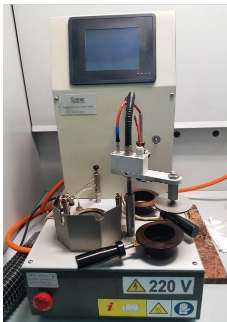
Fig. 2. Scavini automatic flash and fire point tester
